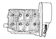
Following sequence above shown, torque engine head nuts twice.
