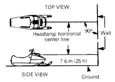
With the suspension correctly adjusted, the rider seated on the vehicle and the high beam ON check that the center of high intensity zone of high beam is 50 mm (2") below horizontal line of headlamp height.
