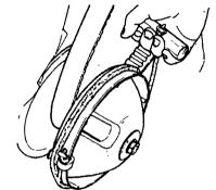
WARNING: Do not wind starting rope around your hand. Hold rope by the handle only.
