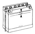
If necessary add distilled water. Battery connections must also be free of corrosion. If cleaning is necessary remove corrosion using a stiff brush then clean with a solution of baking soda and water. Rinse and dry well.
