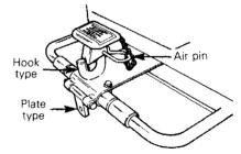
Fixed on the rear bumper, the hitch has two attachment points. A hook type and a plate type. A hair pin is supplied to lock the hook type attachment.
