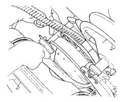
WARNING: Never start or run engine without the drive belt installed. Running an unloaded engine is dangerous.
