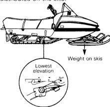
At the highest position the weight is transferred to the track. The rear adjuster blocks should be adjusted to suit the driver's preference.
