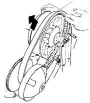
4. Lift the countershaft upward approx. 50 mm (2 in.) and slip the belt between the shaft and the bearing cage to remove completely.
