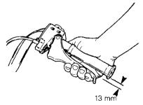
If adjustment is required, turn the brake cable adjuster counter-clockwise until the brake disc is hard to turn then back off the adjuster to approximately 1/2 turn. Recheck brake operation.
