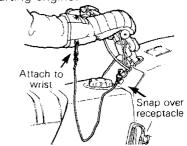
If emergency engine "shut off" is required, completely pull cap from safety switch and engine power will be automatically shut "off".
