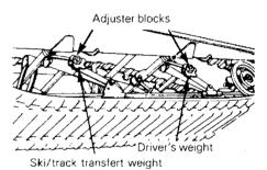
When the front adjuster blocks are at the lowest elevation more weight is distributed on the skis.
