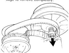
NOTE: It may be necessary to loosen the brake adjustment in order to easily lift the countershaft.
