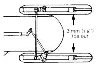
The handlebar should also be horizontal when the skis are pointed toward the front.
