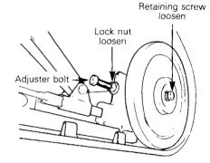
NOTE: Track tension and alignment are inter-related. Do not adjust one without the other.
