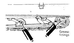
Also lubricate front & rear arms on models equipped with grease fittings.
