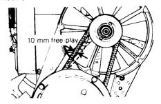
If belt seems damaged or if tension is incorrect, contact your dealer immediately.
