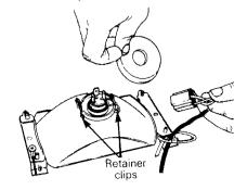
If taillight bulb is burnt, expose the bulb by removing the red plastic lens. To remove, unfasten the two (2) screws.
